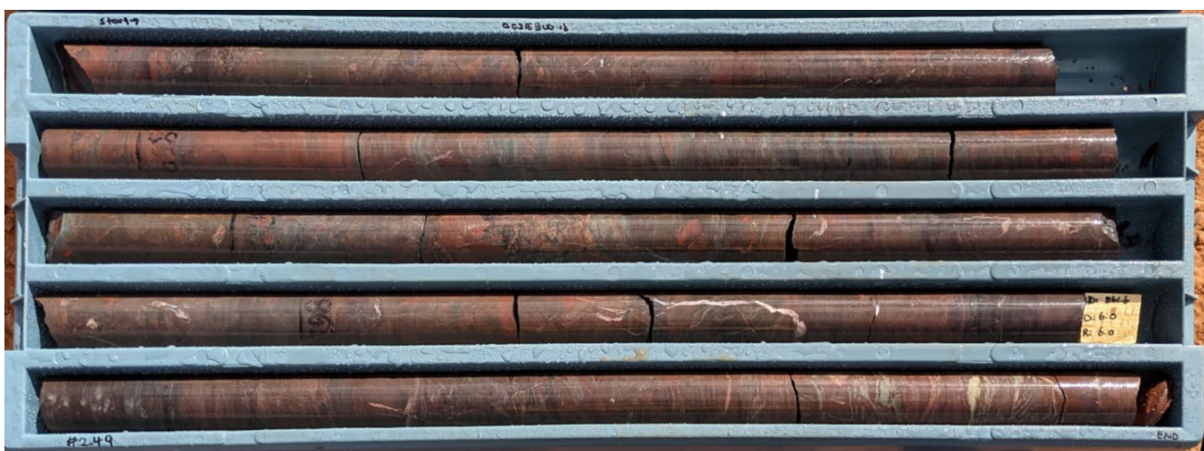
Figure 14 Below the zone of most intense copper sulphide mineralisation, silica alteration begins to dominate.
