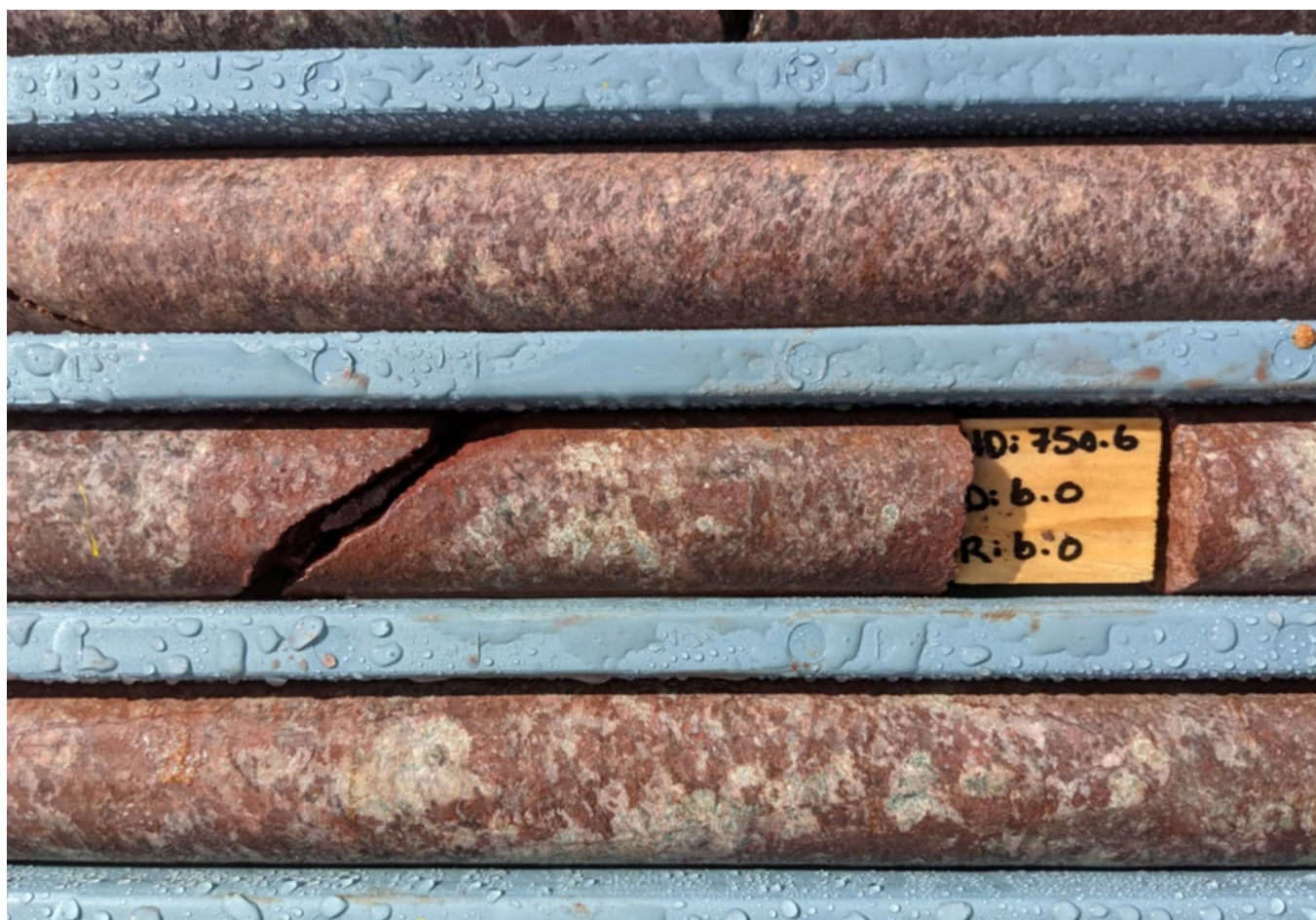
Figure 10 Closeup showing texture and alteration patterns in the Hiltaba Suite granite.
