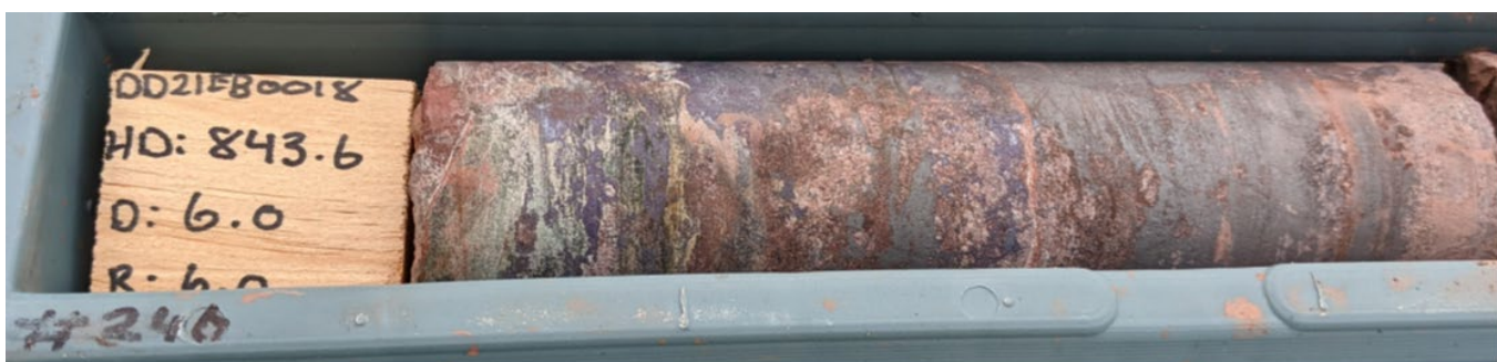
Figure 13 Closeup of core within the copper mineralised zone from 843.6m showing prominent bornite. Bornite is located in small blebs and veinlets throughout the intensely altered zone, but is most prevalent in the lower several metres, proximal to the zones of most intense silicification.
