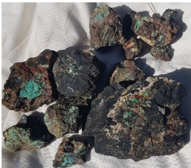
Figure 1 Sample R21CR0143, bleached and altered Corella Formation calcareous siltstone with malachite and minor azurite, collected 250m east of the Rebound prospect. Returned assays of 2.74g/t Au, 156g/t Ag, 9.15% Cu.
